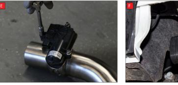
Once happy with fitment of Scorpion Exhaust, fully tighten up all clamps and fixing and plug in the electronic valve
